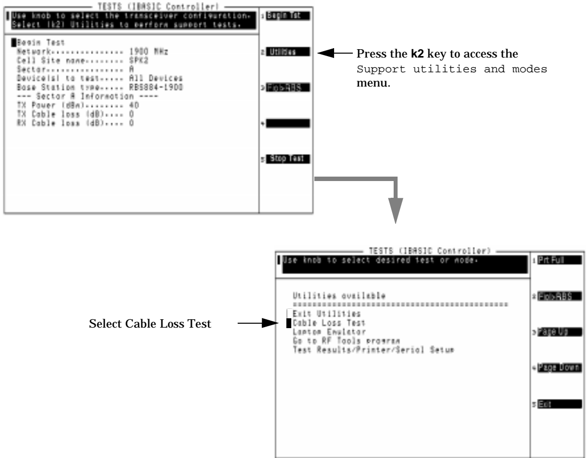
Figure 3-2 Accessing the Cable Loss Test
