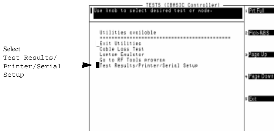
Figure 6-44 Accessing the Settings for Disabling Data Logging
