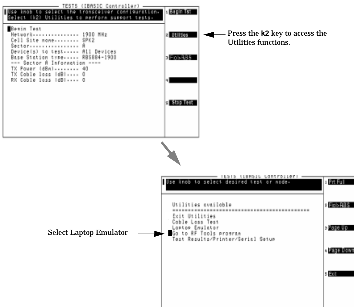
Figure 3-8 Accessing the Laptop Emulator from the Cell Site Information Menu
